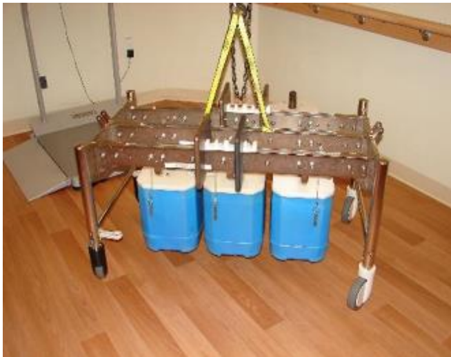
Figure 1: Standard Lift Load
